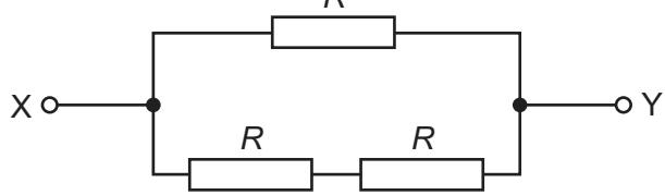
The total resistance between points X and Y is  $8.0\Omega$ .
