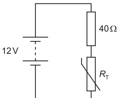
Initially, the temperature of the thermistor is  $15^\circ\text{C}$  and the current in the circuit is 0.10 A.
